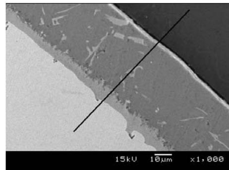
**Fig 6: Aluminium Coated-Riviersonderend**
