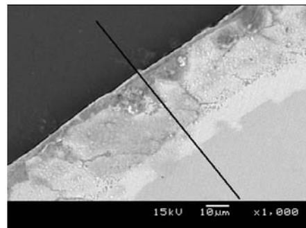
**Fig 2: Heavy Galvanized-Riviersonderend**
