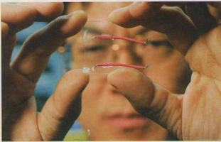
threads are moved relative to each other the friction causes the crystals to bend, generating electricity. The gold-coated thread carries away the electricity, which could be stored or used to power small electronic
